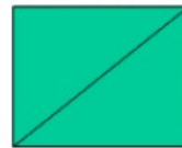
A quad Decomposed into 2 triangles for FEM models
